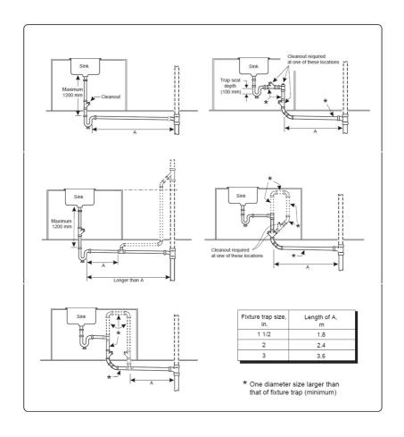
Figure A-2.4.8.2.(1) Island Fixture Installation.
