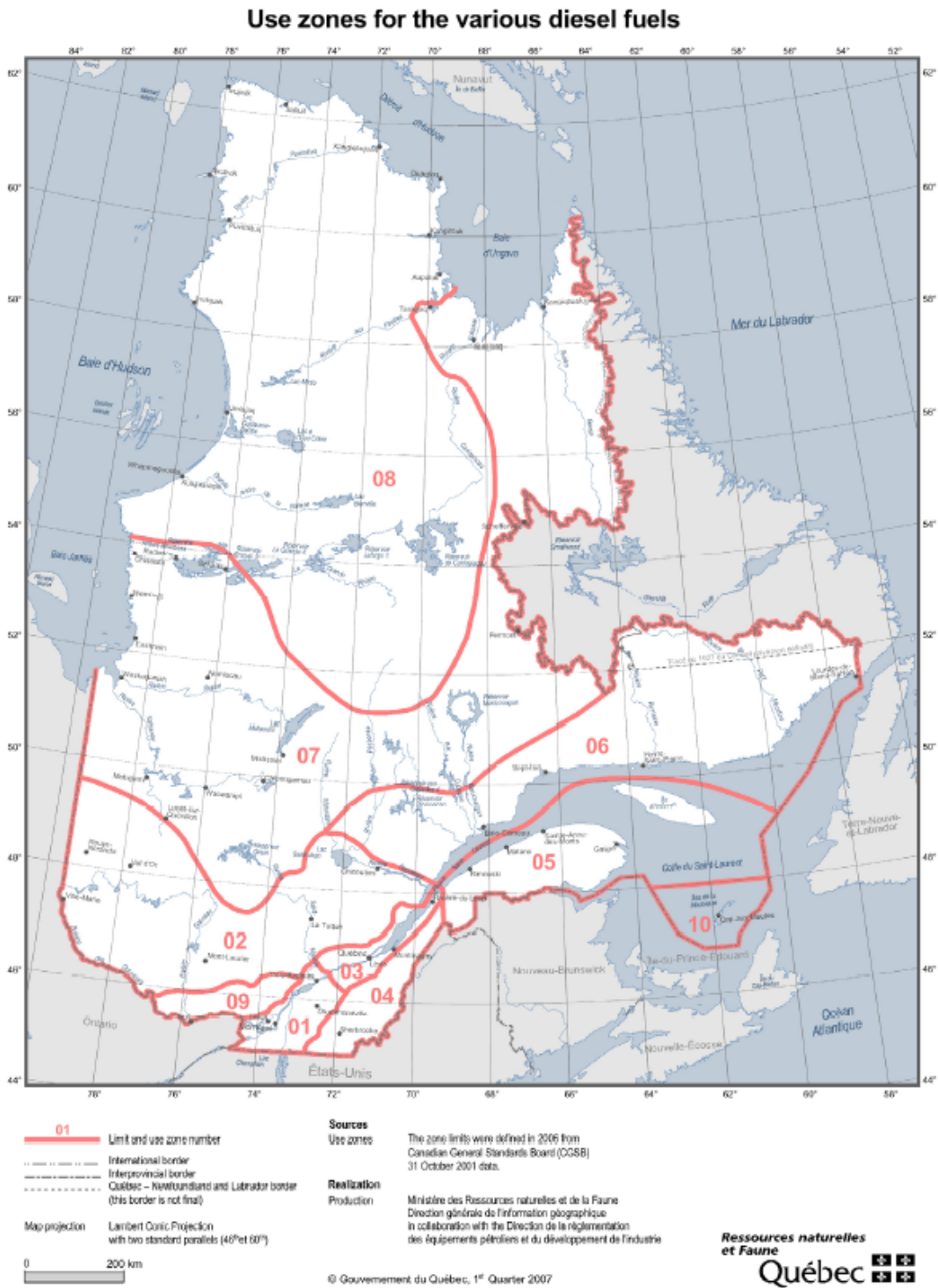
MAP ILLUSTRATING THE LIMITS OF USE ZONES OF DIESEL FUELS ACCORDING TO THE AVERAGE 2.5% LOW-END DESIGN TEMPERATURES
